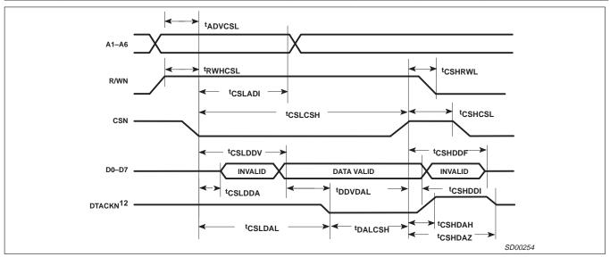
Figure 2. Read Cycle Bus Timing
