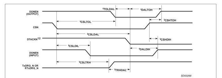
Figure 14. Transmit, Dual Address DMA
