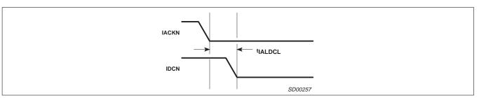
Figure 5. Interrupt Daisy Chain Timing
