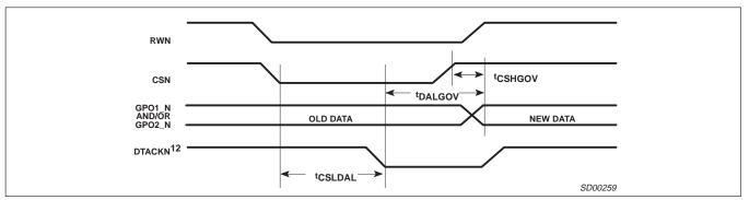
Figure 7. Output Port Timing
