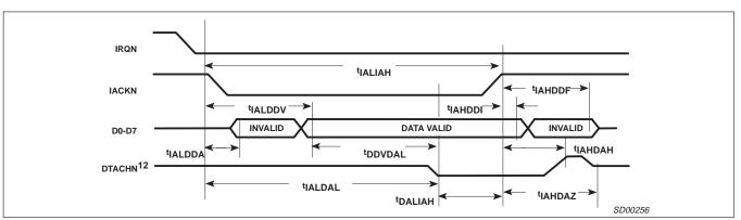
Figure 4. Interrupt Cycle Timing
